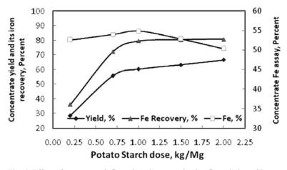
Fig. 6. Effect of potato starch flocculant dose on selective flocculation of iron ore (feed size, 100% - 0.075 mm, pH = 10.5, sodium silicate dose 1 kg/Mg, and flocculation S/L ratio = 5)
