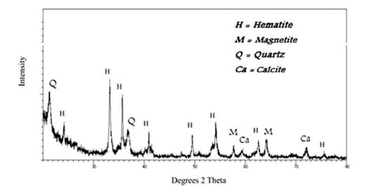
Fig. 2. XRD pattern of the "as received" powdered iron sample
