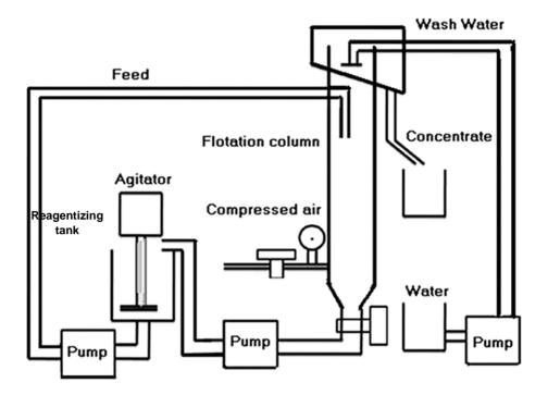
Fig. 1. Experimental setup for column flotation of the tested iron ore
